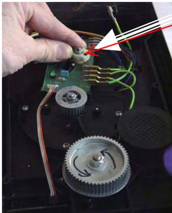
Should the ~~white plastic speed pulser~~ (sits on the pcb at the back) turn as well, just hold it in place with your free hand
