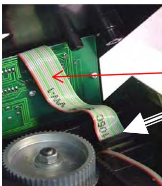
**Do not unplug** the flat band (ribbon) cable. Let the top cover hang from this cable, alongside of the metal housing (casing).
