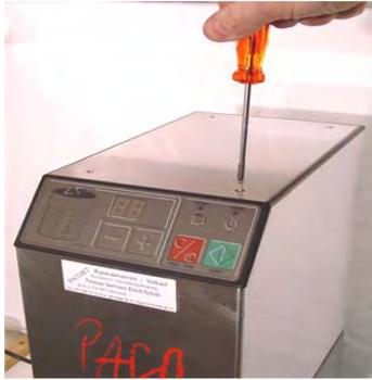
**Remove** metal top plate (4 screws)
