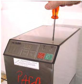
**Remove** metal top plate (4 screws)
