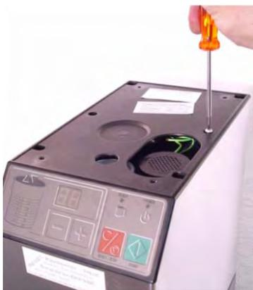
**Remove the 6 sunken screws of black plastic top cover.**
